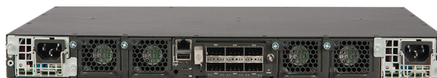
Figure 5: The Ruckus ICX 7750 features hot-swappable redundant power supplies (1+1) and fans (3+1), and an optional 6 40 GbE ports module that can be used for stacking or as additional 40 GbE data ports.
