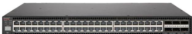
Figure 2: The Ruckus ICX 7750-48C features 48 10GBASE-T ports and 6 40 GbE QSFP+ ports that can each be split* into 4x10 GbE SFP+ ports.
