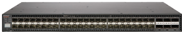
Figure 1: The Ruckus ICX 7750-48F features 48 1/10 GbE SFP+ ports and 6 40 GbE QSFP+ ports that can each be split* into 4x10 GbE SFP+ ports. The front panel also displays the unit stacking ID.
